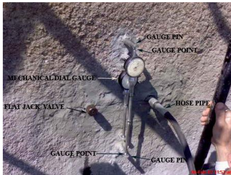
Figure 14. View of embedded flat jack and four reference pins in the slot.
