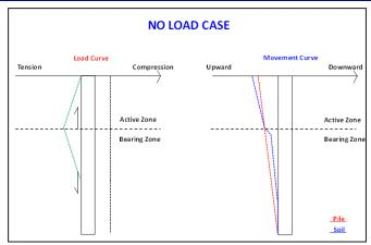
Fig. 1 – Load in drilled shaft – no load case.
