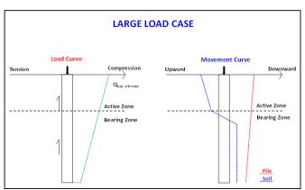
Fig. 2 – Load in drilled shaft – large compression load case.
