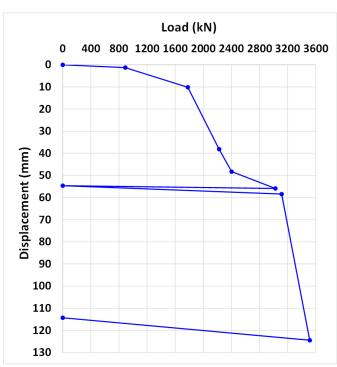
Fig. 4 – Johnson and Stroman (1982) case history: (a) dimensions of pile LAFB-2 and stratigraphy, (b) load test result (Johnson, 1984).
