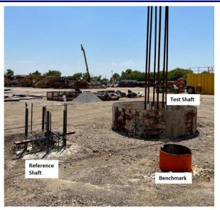
Fig. 13 – Test set up.
