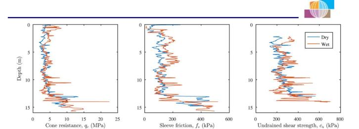
Fig. 7 - CPT results and inferred undrained shear strength (Da Silva Burke et al., 2022).
