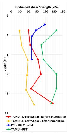
Fig. 11 – Undrained shear strength results.
