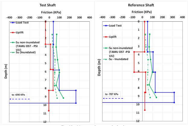
Fig. 18 – Maximum friction on both piles.
