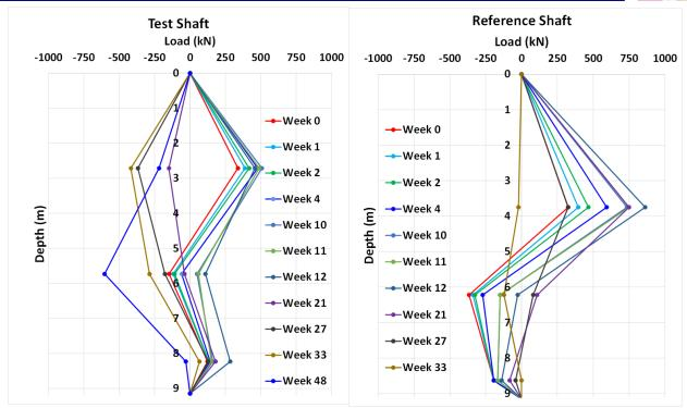
*Fig.* 15 – Load distribution in both piles.
