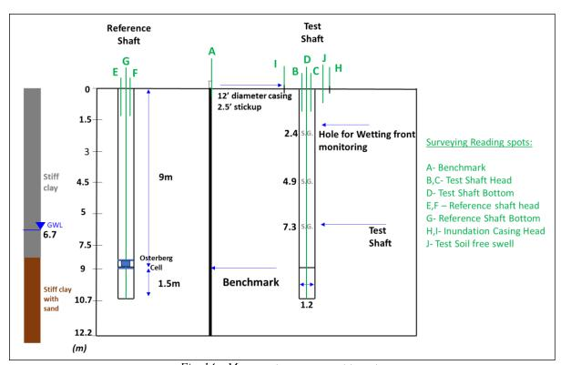
Fig. 14 – Movement measurement targets.
