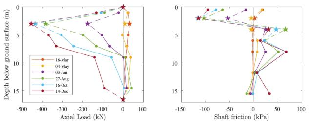
Fig. 9 – Compression load in the non-inundated reference pile (Da Silva Burke et al., 2022).
