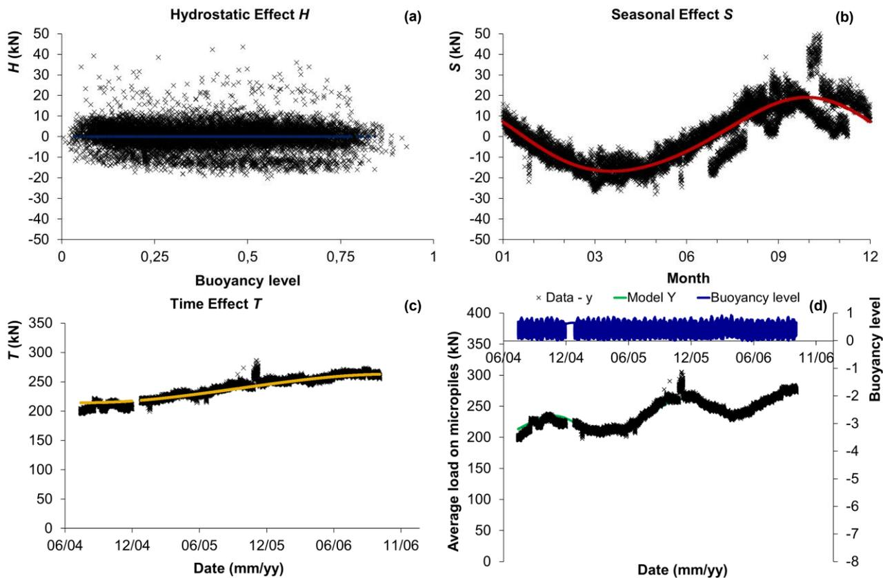
Figure 18. Results of HST analysis of P01 measurements in 2004-06 (after reinforcement):
