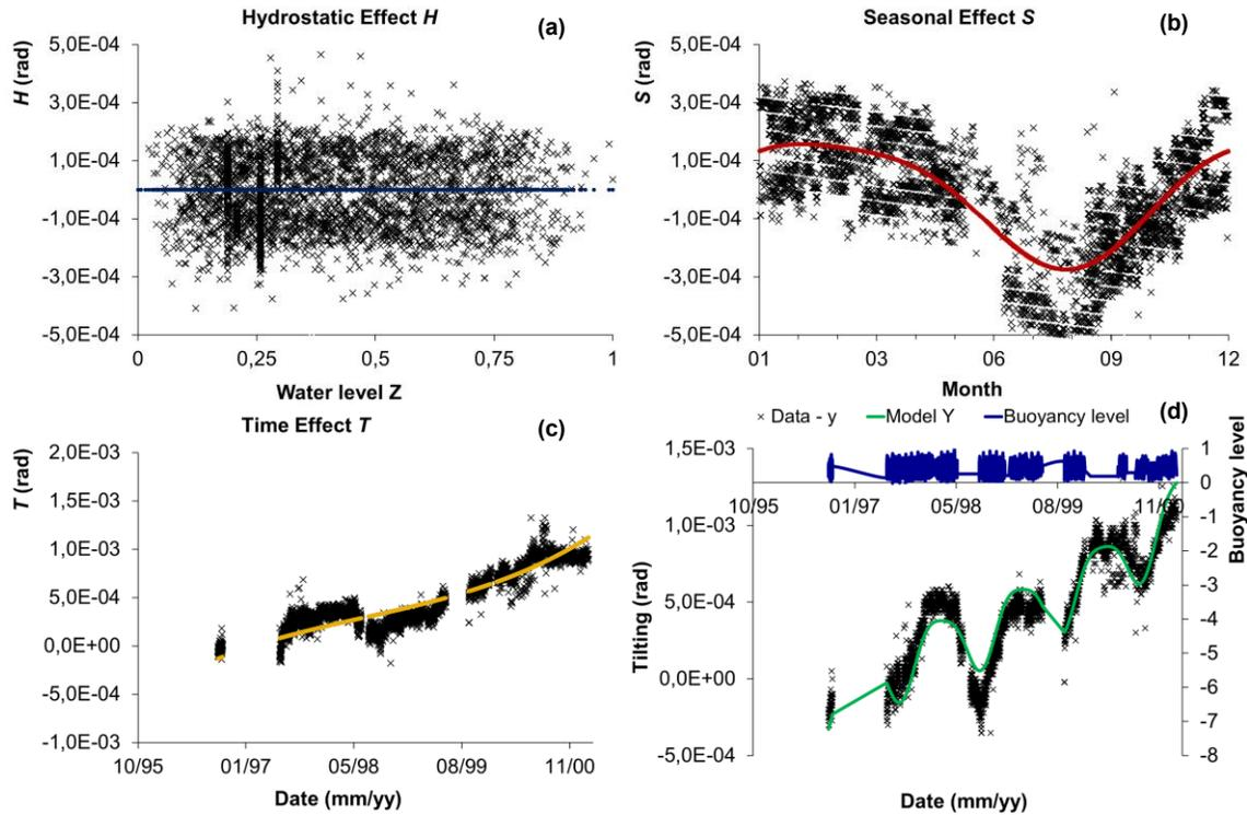
Figure 12. Results of the HST analysis of P06 measurements in 1992-2002 (before reinforcement): (a) Hydrostatic effect  $H$ , (b) Seasonal effect  $S$ , (c) Time effect  $T$ , and (d) Data, model and buoyancy level.
