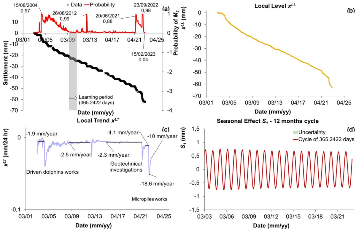
Figure 23. Results of OpenBDLM analysis of P08 measurements in 2003-23: (a) Data and probability of abnormal Model  $M_2$ , (b) Local level  $x^{LL}$ , (c) Local trend  $x^{LT}$ , and (d) 364.2422 days cycle  $S_1$ .
