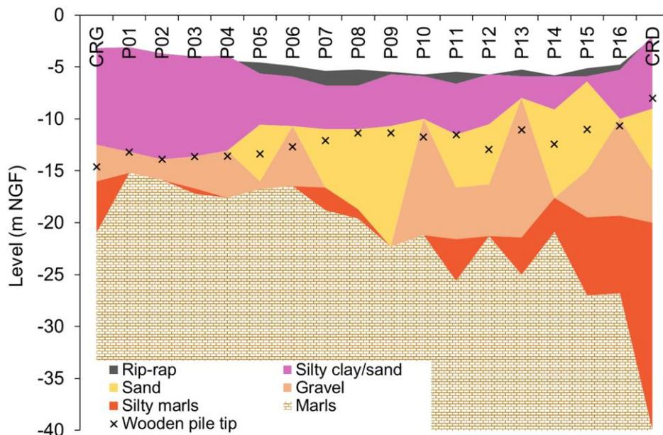
Figure 2. Geotechnical longitudinal profile.
