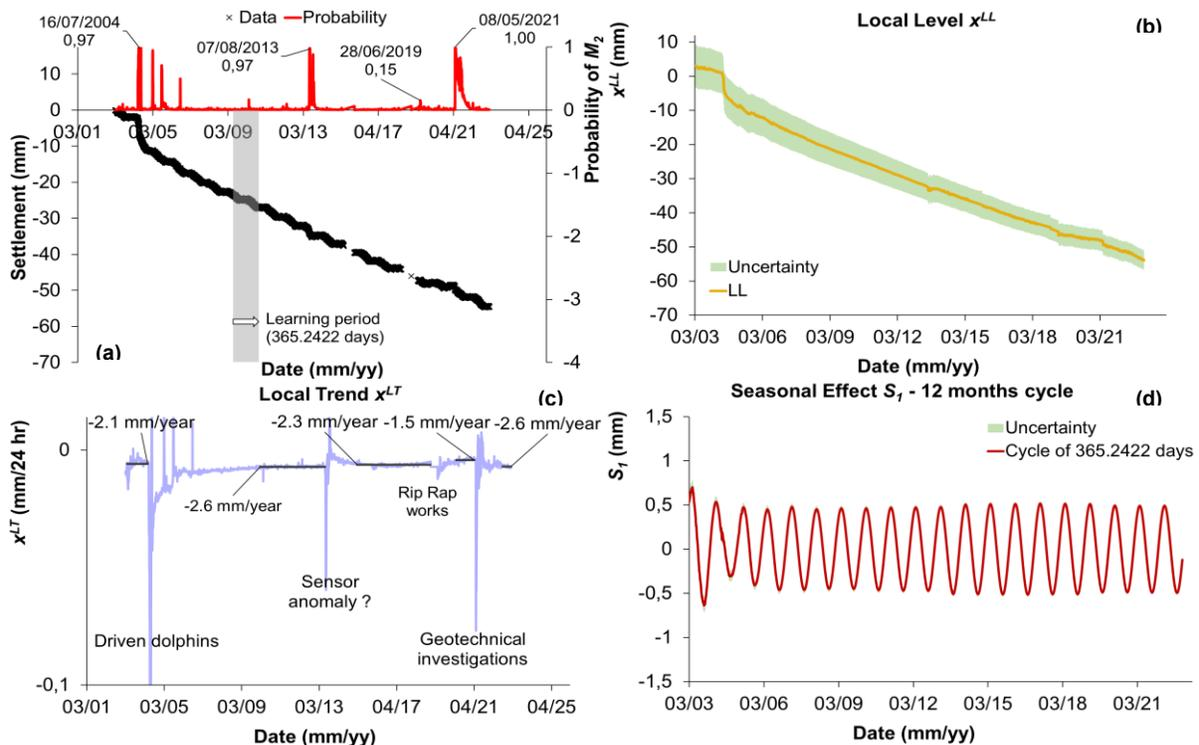
Figure 24. Results of OpenBDLM analysis of P09 measurements in 2003-23: (a) Data and probability of abnormal Model  $M_2$ , (b) Local level  $x^{LL}$ , (c) Local trend  $x^{LT}$ , and (d) 364.2422 days cycle  $S_1$ .
