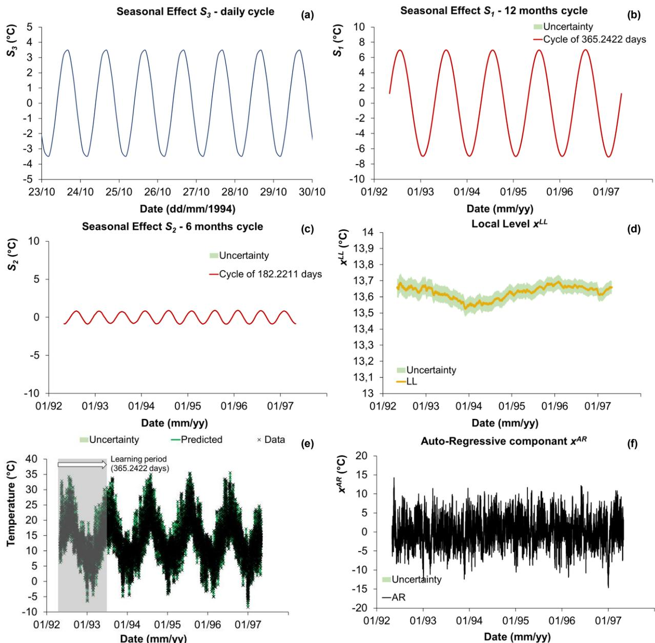
Figure 16. Analysis of meteorological data with OpenBDLM in 1992-97: (a) Daily effect  $S_3$ , (b) Seasonal effect 364.2422 days cycle  $S_1$ , (c) Seasonal effect 182.2211 days cycle  $S_2$ , (d) Local Level  $x^{LL}$ , (e) Datas and model, and (f) Auto-Regressive  $x^{AR}$  component.
