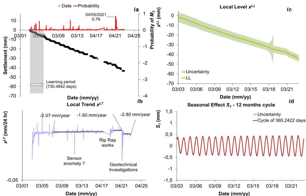
Figure 22. Results of OpenBDLM analysis of P07 measurements in 2003-23: (a) Data and probability of abnormal Model  $M_2$ , (b) Local level  $x^{LL}$ , (c) Local trend  $x^{LT}$ , and (d) 364.2422 days cycle  $S_1$ .
