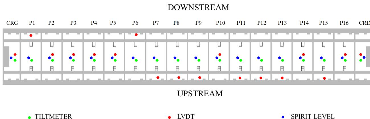
Figure 5. Schematic of sensor layout on the bridge.
