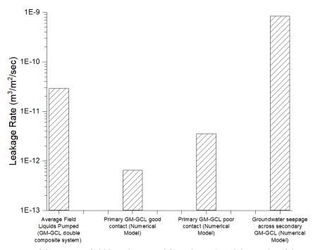
Figure 9. Comparison of the average field liquids pumped from the LDS and the results of the numerical model.
