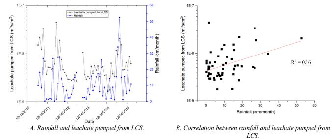
Figure 3. A graph of rainfall recorded at the landfill site and leachate pumped from the leachate collection system (LCS), and a graph of the correlation between rainfall and leachate pumped from the LCS.
