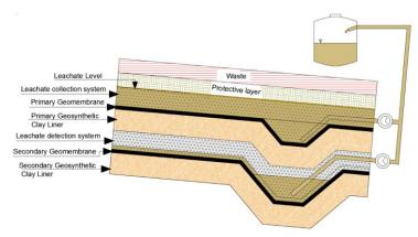
Figure 2. Schematic drawing of the cross-section of the GM-GCL double composite lining system for the landfill (Cell 1).
