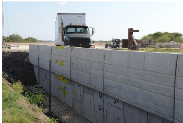
Figure 12. Test set up just before impact test.
