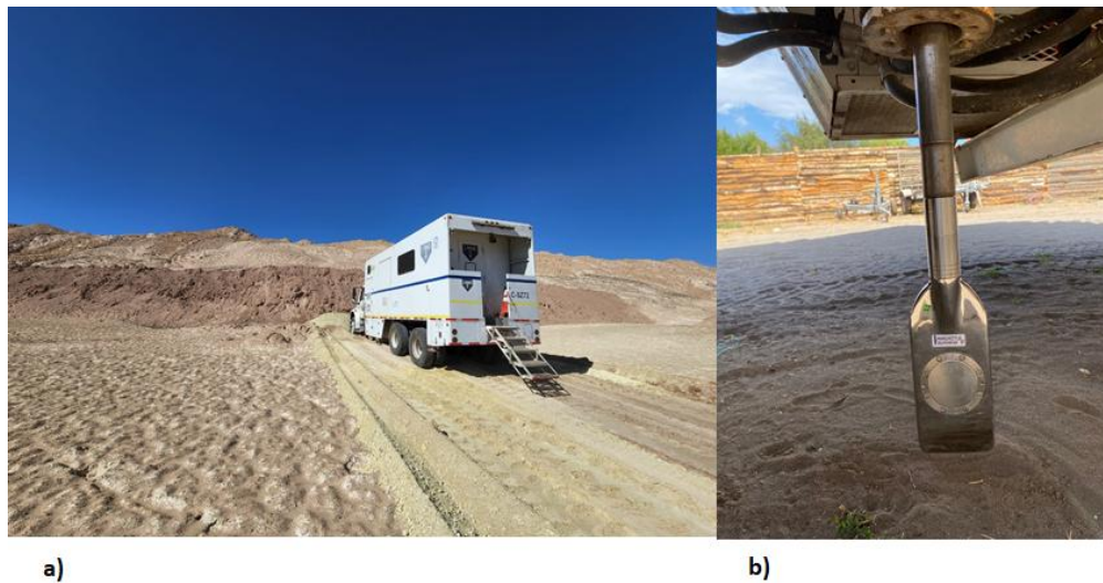
Figure 3. In-situ testing: a) CPT truck, b) DMT probe.
