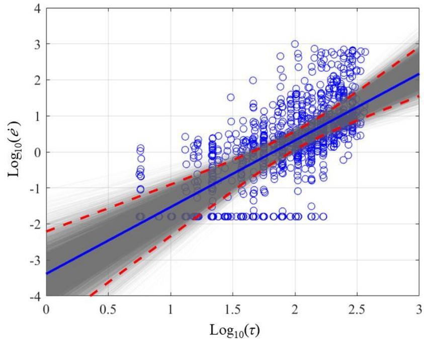
Figure 11. Bootstrapping technique showing 50,000 linear fittings, Source: FHWA.
