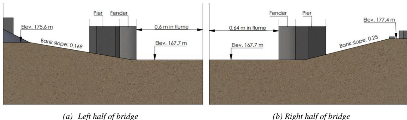
Figure 13. Scaled bridge models in MFS, Source: FHWA.
