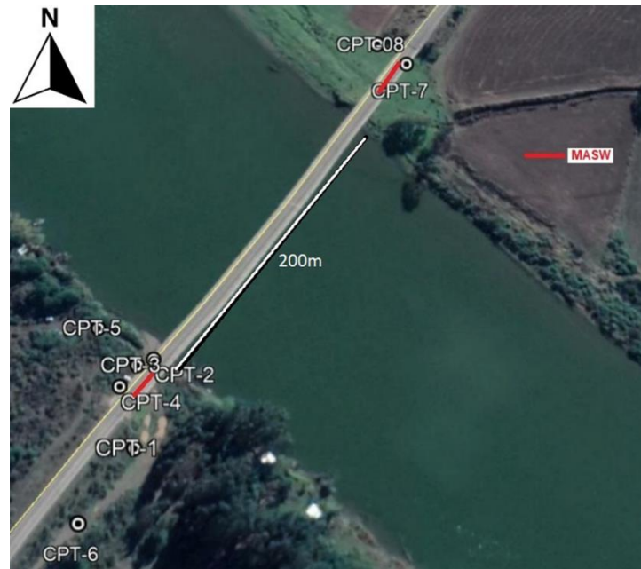
Figure 11. Posterior subsurface investigation locations from the 2019 field campaign.
