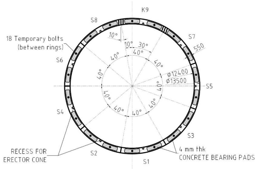
Figure 10. Segmental tunnel linings (dimension in mm).
