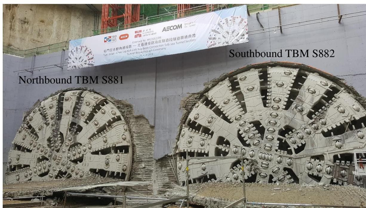
Figure 9. 14 m diameter slurry mix-shield TBMs.
