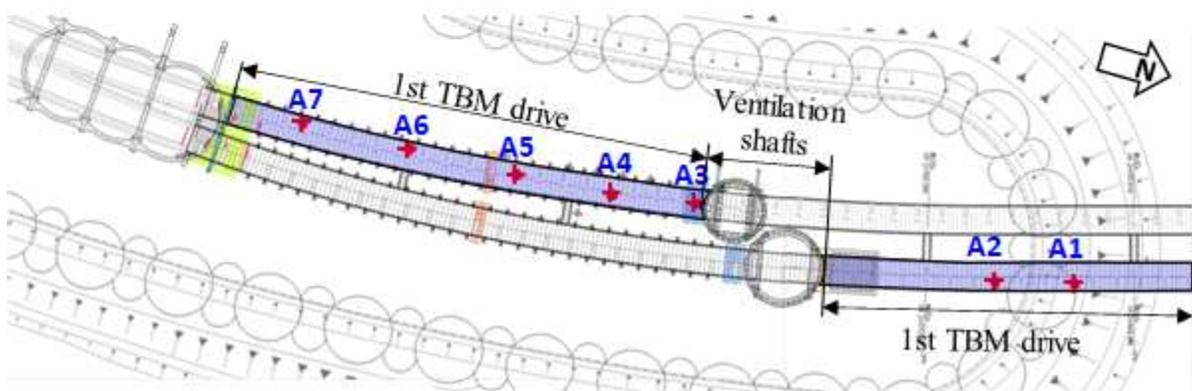
Figure 18: Tunnelling-induced consolidation settlements after 1<sup>st</sup> TBM drive.
