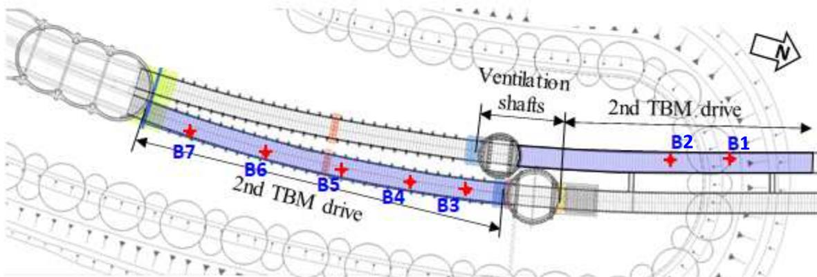
Figure 19: Tunnelling-induced consolidation settlements after 2<sup>nd</sup> TBM drive.
