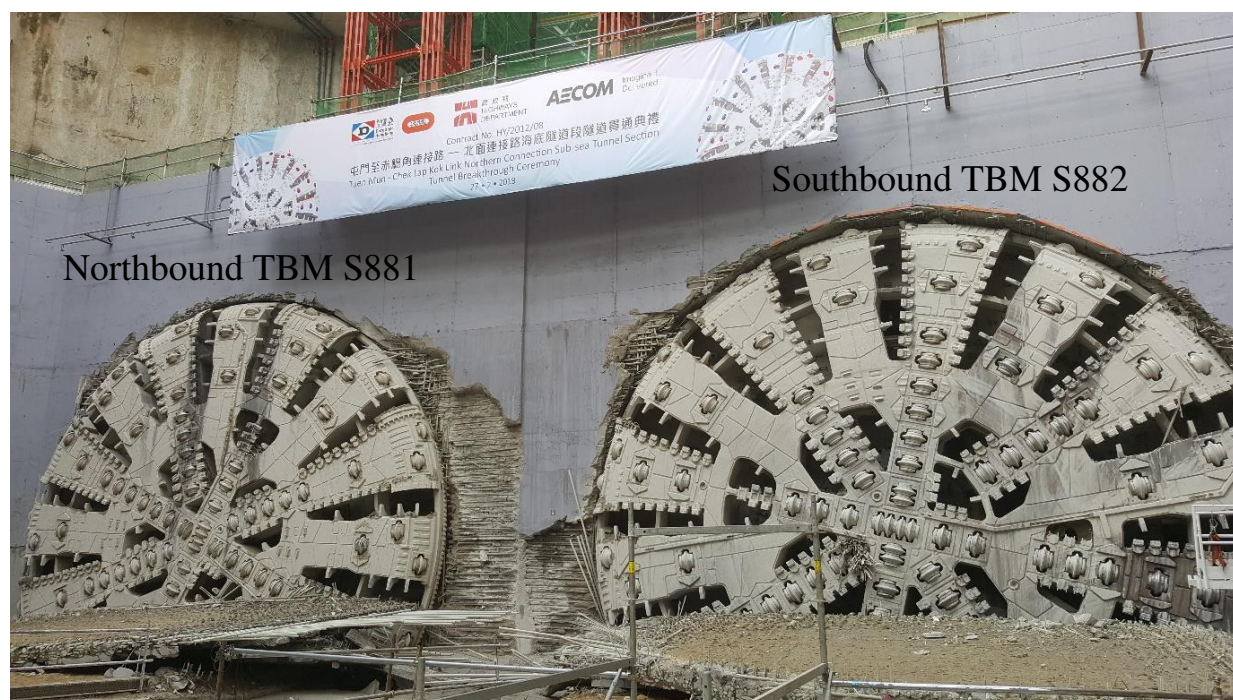
Figure 9. 14 m diameter slurry mix-shield TBMs.
