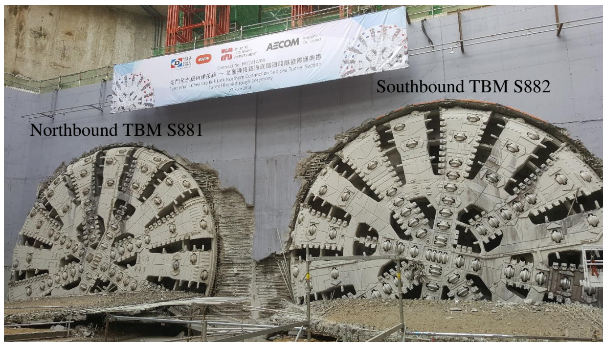
Figure 9. 14 m diameter slurry mix-shield TBMs.
