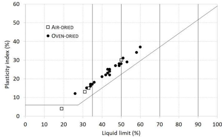
Figure 4(a). Alluvial clay – Casagrande plasticity chart.
