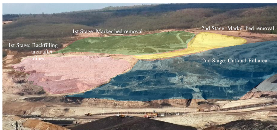
(c) Marker bed removal and 2 nd Stage preparation in 1 st Stage (as of April 2014)
