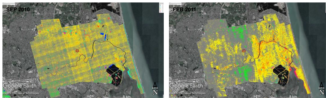
Figure 8. Vertical Ground Movements (adjusted for the tectonic component) for the Sep 2010 and Feb 2011 earthquakes (CGD, 2012b) – the site is in the zone of overestimated ground surface subsidence for the Sep 2010 earthquake and the zone of underestimated ground surface subsidence for the Feb 2011 earthquake.
