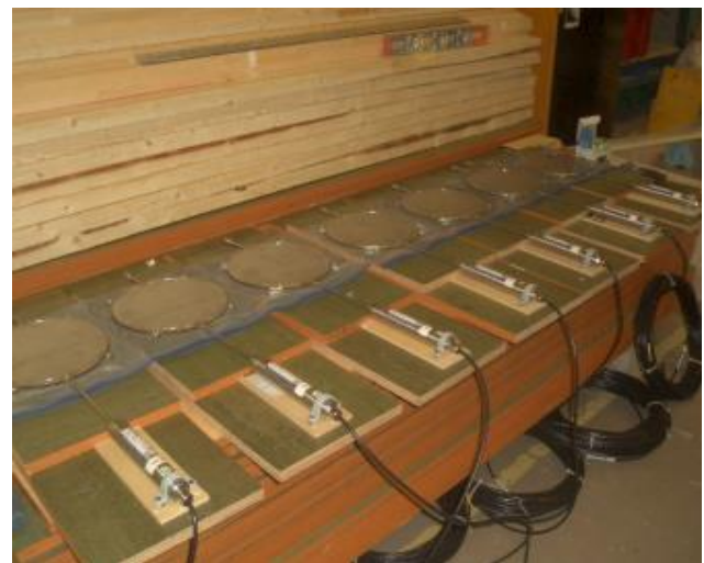
(d) Sufficient sensor cables were attached to each pressure cell for extra length if required to connect with the SENSLOG.
