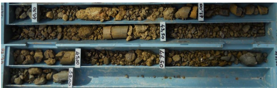
Figure 7. Very weathered GREYWACKE.
