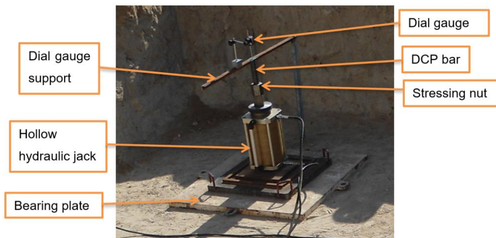
Figure 51. Typical arrangement of acceptance test.
