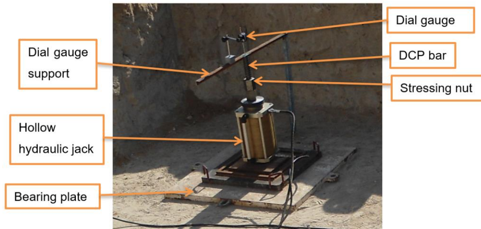
Figure 51. Typical arrangement of acceptance test.
