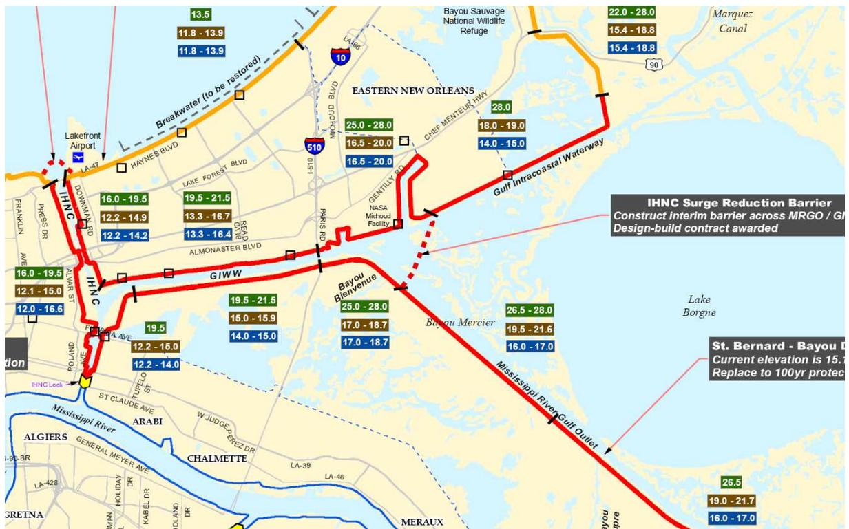
Figure 2. Section of HSDRRS plan, eastern New Orleans and St. Bernard Polders. ([http://www.mvn.usace.army.mil/hps/pdf/2008\\_Storm\\_Vulnerability\\_Elev\\_final.pdf](http://www.mvn.usace.army.mil/hps/pdf/2008_Storm_Vulnerability_Elev_final.pdf))
