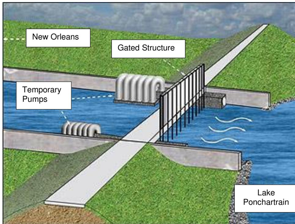
Figure 7. Schematic of canal closure facilities .([http://www.mvn.usace.army.mil/hps2/hps\\_outfall\\_canals.asp](http://www.mvn.usace.army.mil/hps2/hps_outfall_canals.asp))
