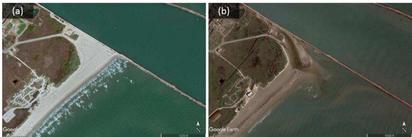
Figure 3. (a) Pre-storm satellite imagery (imagery date February 22, 2017) and (b) post-storm satellite imagery (imagery date August 29, 2017) show the eroded runnel created during Hurricane Harvey near Port Aransas Pass (location 27^{\circ}50'6.39''N , 97^{\circ}2'50.56''W ). Map data: Google Earth, Digital Globe.
