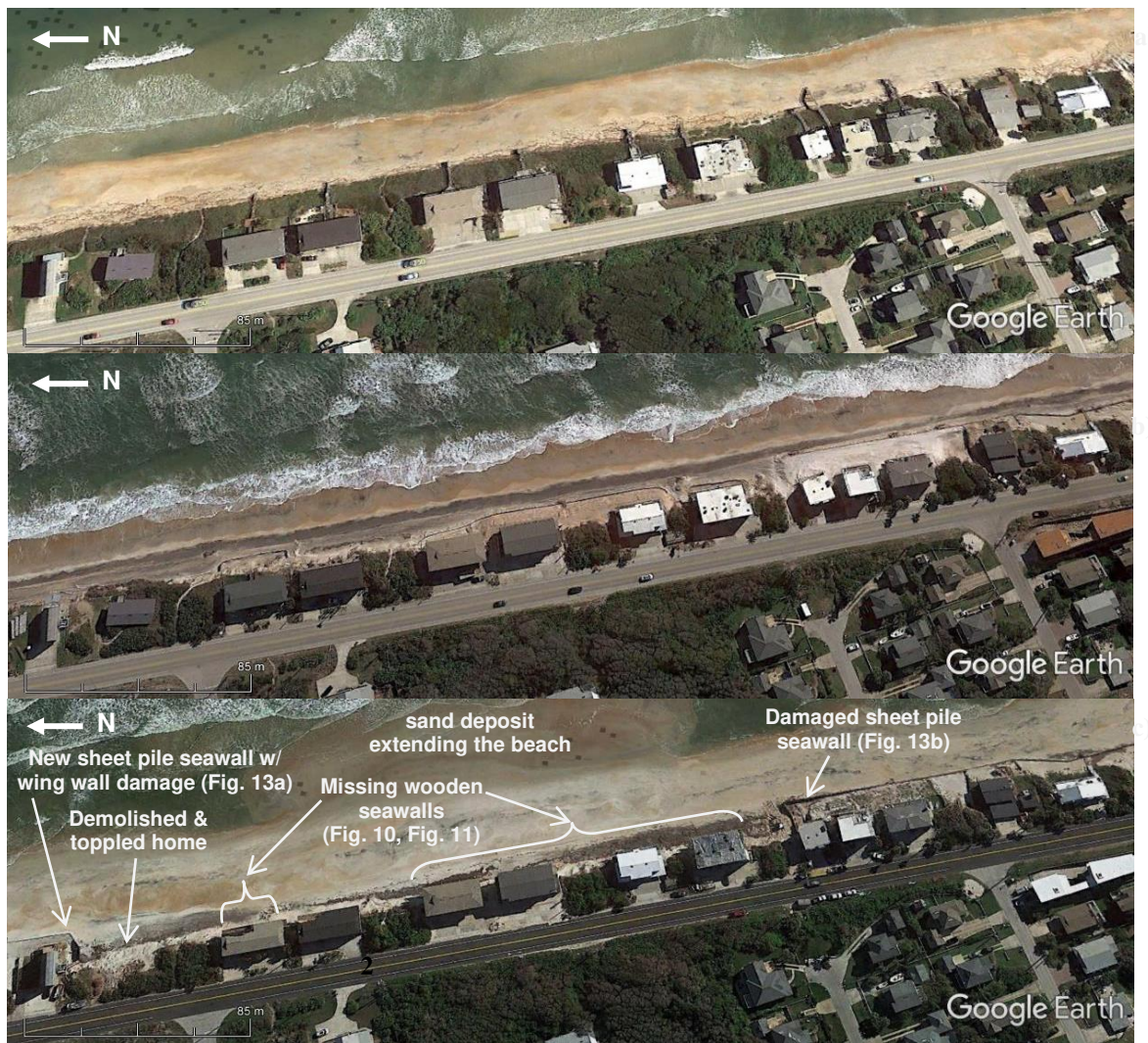
Figure 9: Changes to the Vilano Beach coastline from 4020 to 3880 Coastal Highway, St. Augustine, Florida, at 29^{\circ}56'49.30''\text{N} latitude and 81^{\circ}18'9.37''\text{W} longitude dated: (a) November 2015, with few seawalls present; (b) March 2017, with seawalls installed following 2016 Hurricane Matthew, and; (c) October 2018, following damage from 2017 Hurricane Irma (Google Earth, 2018).
