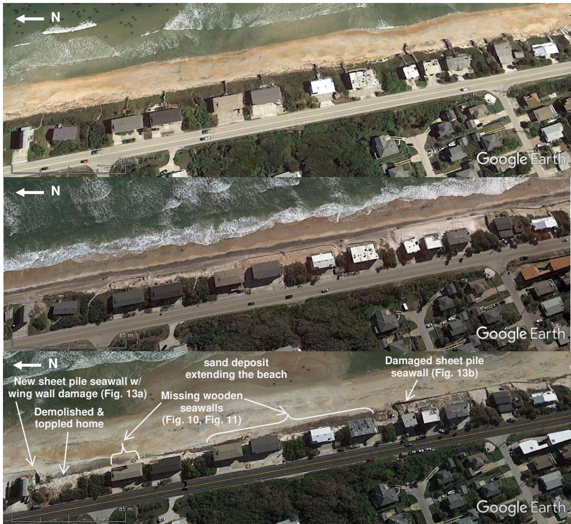
Figure 9: Changes to the Vilano Beach coastline from 4020 to 3880 Coastal Highway, St. Augustine, Florida, at 29°56'49.30"N latitude and 81°18'9.37"W longitude dated: (a) November 2015, with few seawalls present; (b) March 2017, with seawalls installed following 2016 Hurricane Matthew, and; (c) October 2018, following damage from 2017 Hurricane Irma (Google Earth, 2018).
