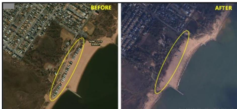
Figure 18. Aerial photographs from New Dorp Beach, SI, before and after Sandy. Row of houses completely removed and debris moved inland. (Images from [tmappsevents.esri.com/website/swipe\\_sandy/](http://tmappsevents.esri.com/website/swipe_sandy/)).
