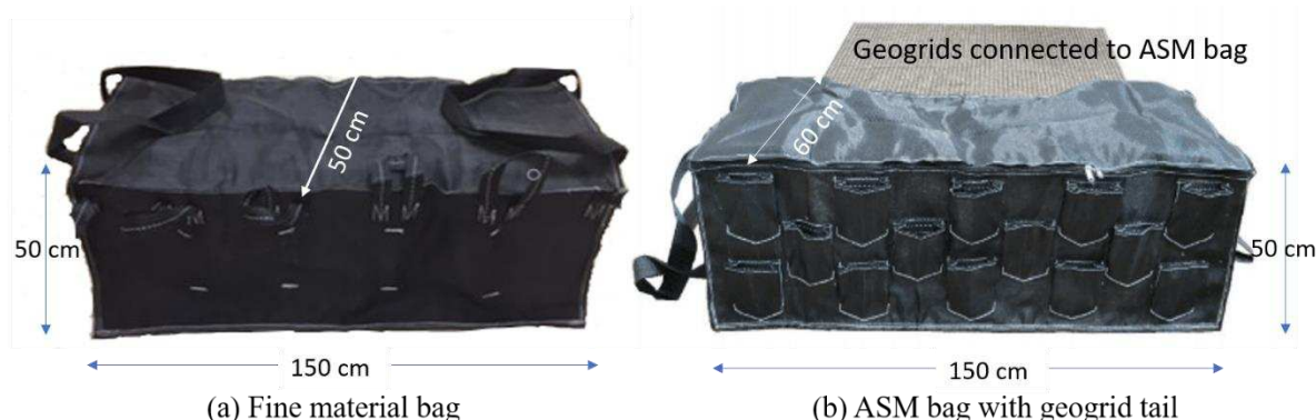
Figure 2. Geotextile bags for fine material and ASM.
