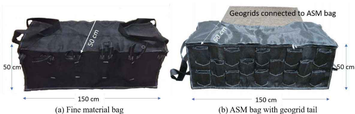
Figure 2. Geotextile bags for fine material and ASM.
