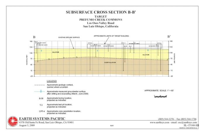
Figure 3. Simplified cross-section profile of the soil conditions at the site.
