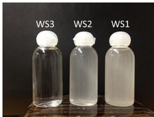
Figure 17. Turbidity of sampled water collected at different point in the Armala area in June 2014 (the water sample locations at ws1, ws2 and ws3 respectively in Figure 2).
