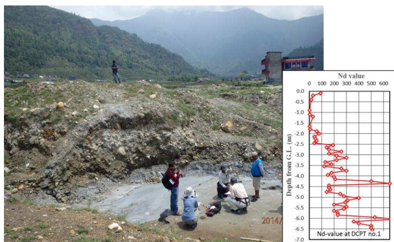
Figure 10. Result of the Dynamic Cone Penetration Test at DCPT no. 1 at the bottom of a sinkhole.
