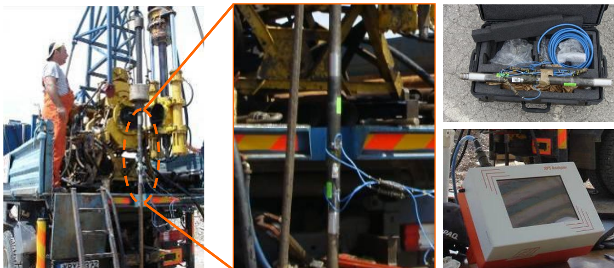
Figure 8. Field energy ratio measurements during SPT testing. (SPT Analyzer, Pile Dynamics Inc.)
