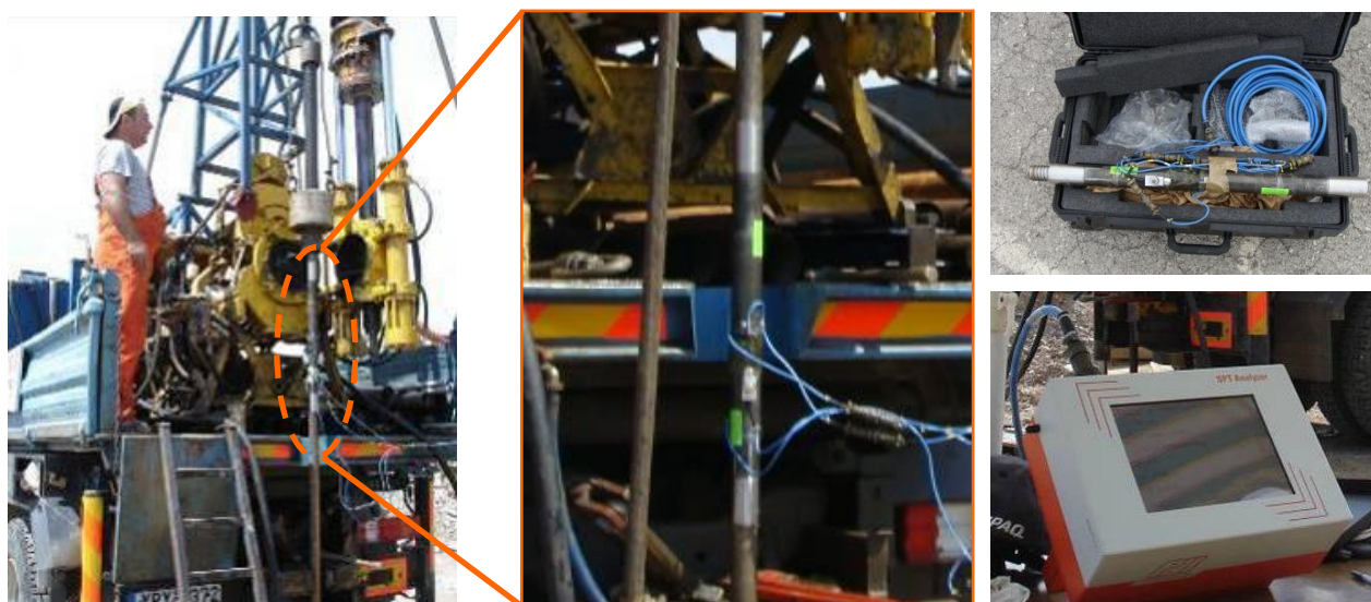
Figure 8. Field energy ratio measurements during SPT testing. (SPT Analyzer, Pile Dynamics Inc.)
