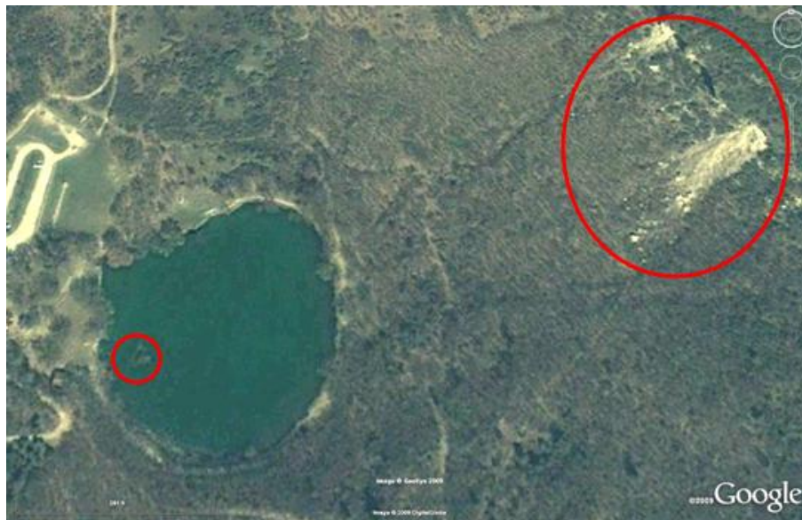
Figure 161. Post earthquake satellite imagery showing submerged trees within small circle and rock slope failures within large circle; compare to pre-earthquake imagery shown in Figure 146 (42.291N 13.576).
