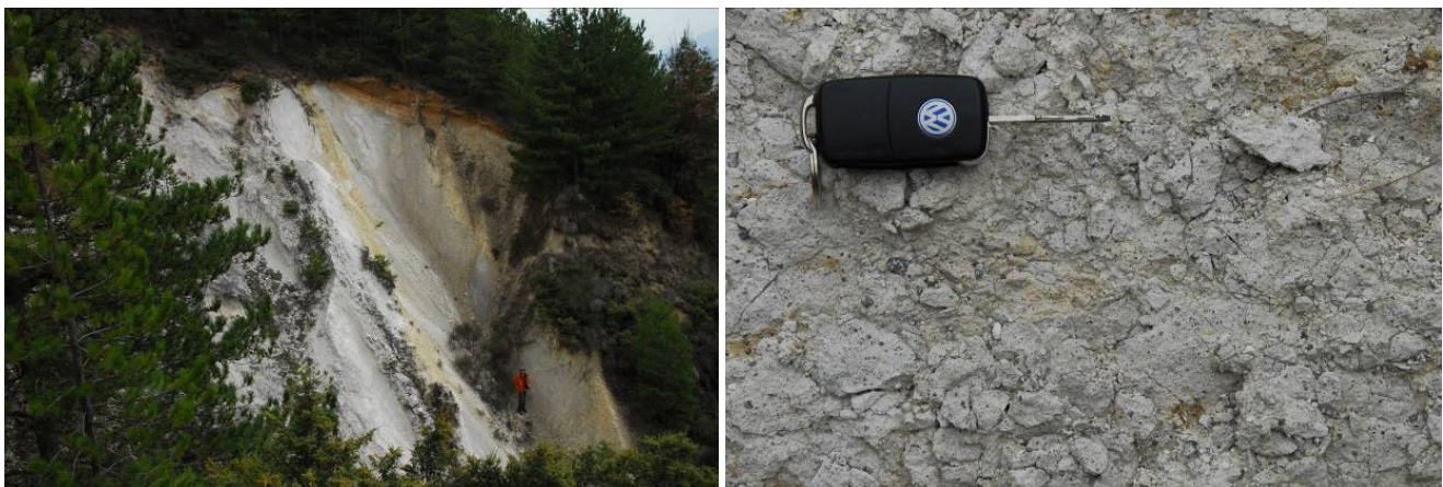
Figure 126. Cataclasite exposed along the Pettino Fault (left) and detail of cemented and interlocked particulate structure (right) (42.376N, 13.365E).
