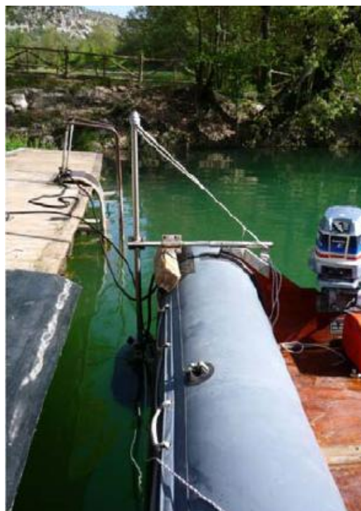
Figure 172. Rubber boat equipped with the 8101 multibeam system.
