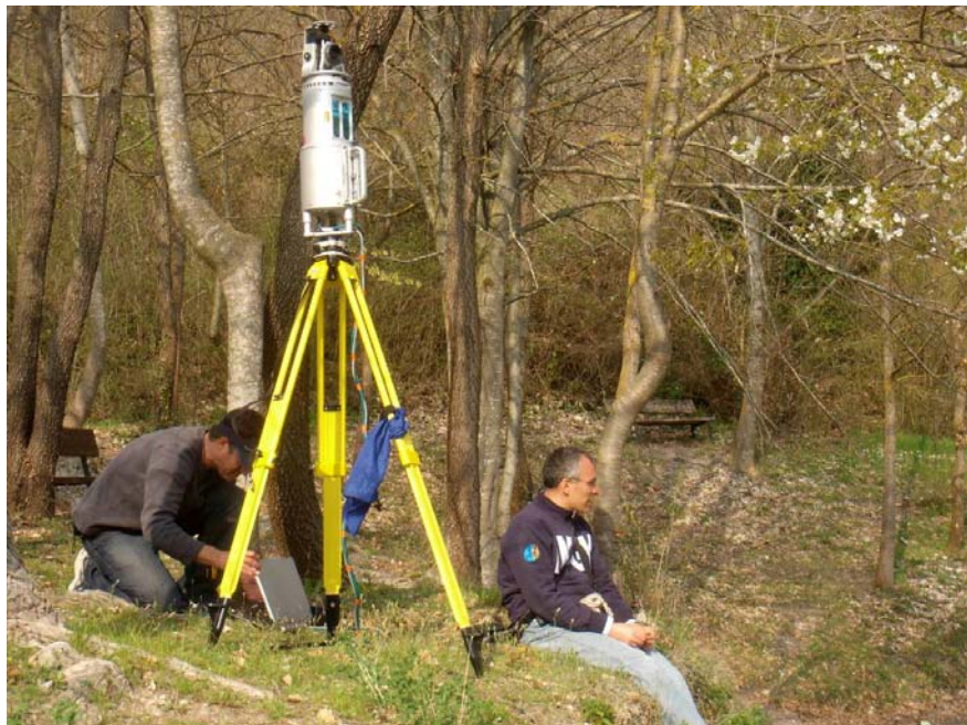
Figure 168. Deployment of the tripod-mounted Lidar system on the lake margin. The laser unit is connected to a laptop, battery, and photogrammetric camera.
