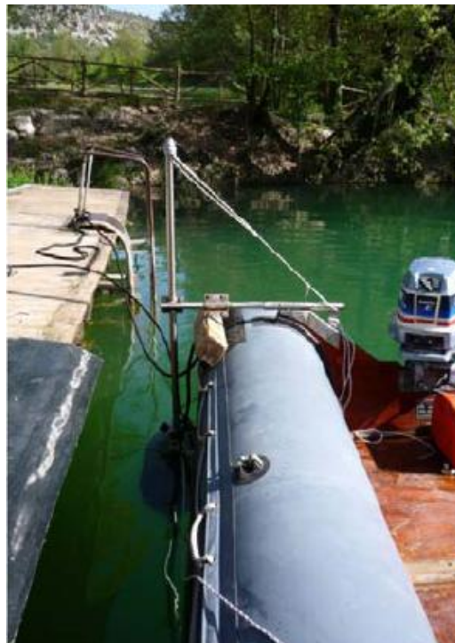
Figure 172. Rubber boat equipped with the 8101 multibeam system.
