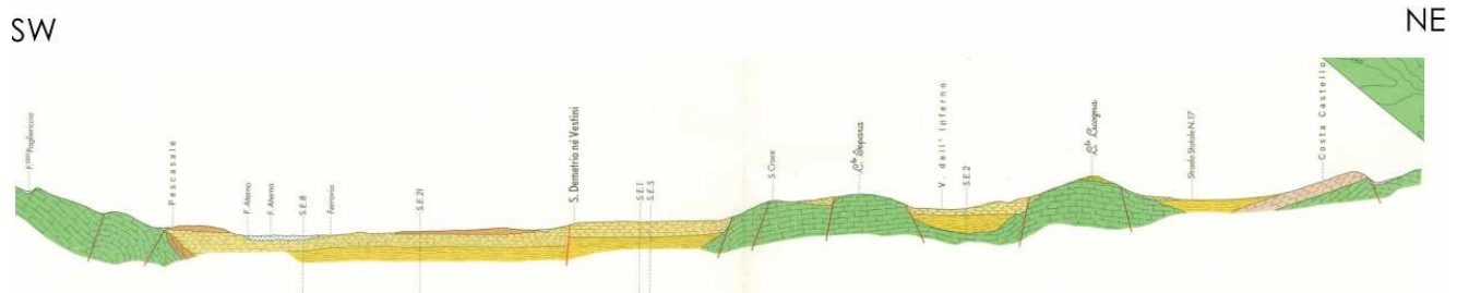
Figure 7. SW-NE Geologic cross-section of the Aterno River Valley (Bosi and Bertini, 1970).
