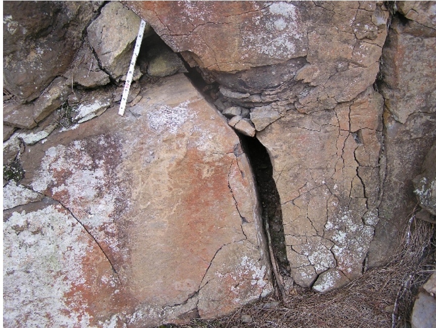
Figure 29. Location 9, Hwy 19 near Honoka'a. Wide fracture likely not caused by earthquake- note debris and tree root.
