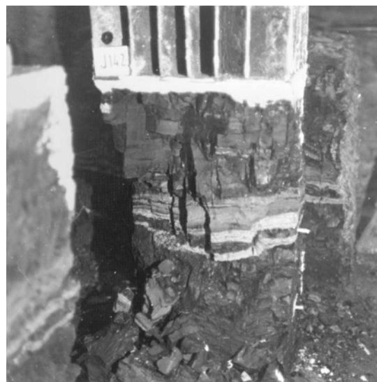
Figure 9. Failed block of coal after testing (Hudek, 1986).
