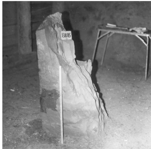
Figure 7. Part of the failed block of the tuffaceous claystone after testing (Hudek, 1986)
