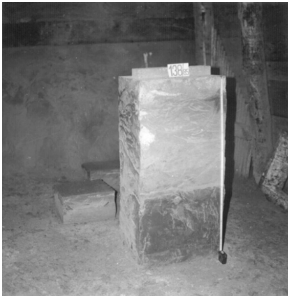
Figure 6. Block of the tuffaceous claystone (0.5 m x 0.5 m x 1.0 m) prepared for an in situ triaxial compression test (Hudek, 1986).
