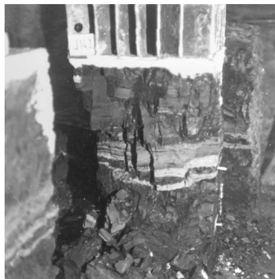
Figure 9. Failed block of coal after testing (Hudek, 1986).
