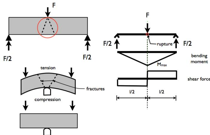
**Figure 6.** Combined extension and shear stress occurs in a beam when the load acts in the middle. This “bending force” produces hybrid fractures, resulting in a triangular or trapezoidal fracture shape (Melvin, 1993).
