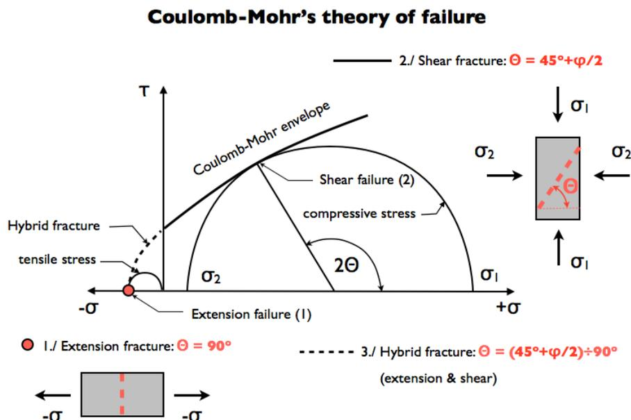
**Figure 4.** The two types of fractures are extension and shear. The dashed line shows the area where hybrid fractures occur, resulting from the transformation from extension to shear failure (Ramsey & Chester, 2004). The angles of the failed surface or fractures are given in relation to the principal stresses for the different failures.
