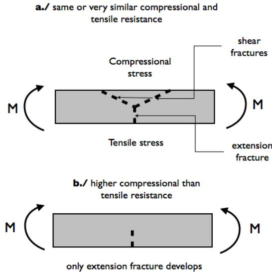
**Figure 5.** The fracture pattern of pure bending is shown. The tensile and compression stresses are on the opposite sides of the beam, developing extension and shear fracture respectively: (a) If the compression and tensile resistances of the substance are the same or similar to each other, then both shear and extension fractures are developing; (b) If the compression resistance of the substance is higher than the tensile resistance, then primarily extension fracture develops.
