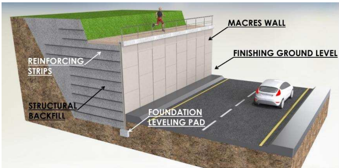
Figure 3. Mechanically stabilized earth wall system.
