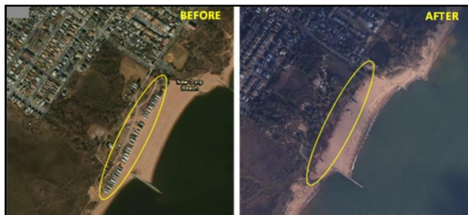
Figure 18. Aerial photographs from New Dorp Beach, SI, before and after Sandy. Row of houses completely removed and debris moved inland. (Images from tmappsevents.esri.com/website/swipe_sandy/ ).
