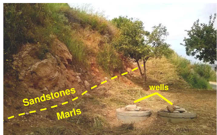
Figure 11. Wells collecting groundwater springing out freely in the sandstone-marl contact area were located a few hundred meters south of the landslide area.
