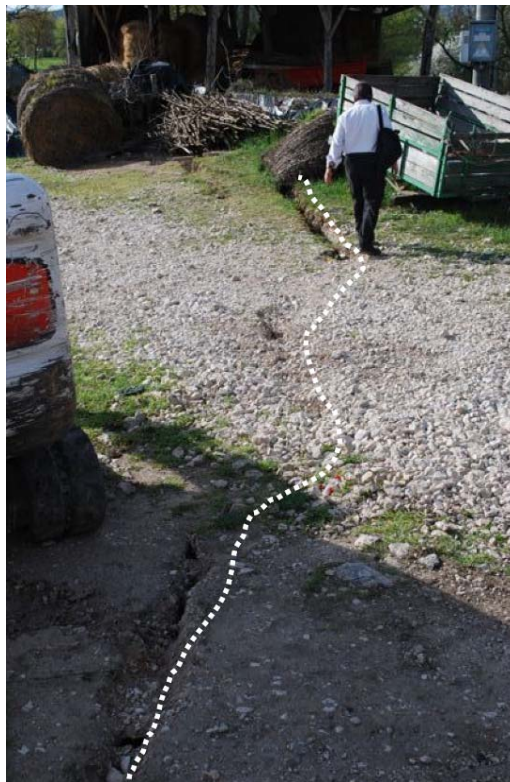
Figure 143. Ground cracks up to 1.0 m deep, 20 m long, and with maximum of 15 cm vertical displacement (down-dropped toward river) developed directly adjacent to bridge abutment (42.324N, 13.478E).
